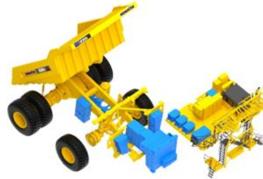
Battery Trolley Configuration
