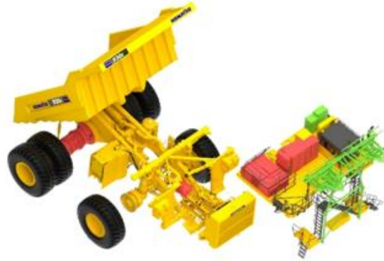
Diesel Trolley Configuration
