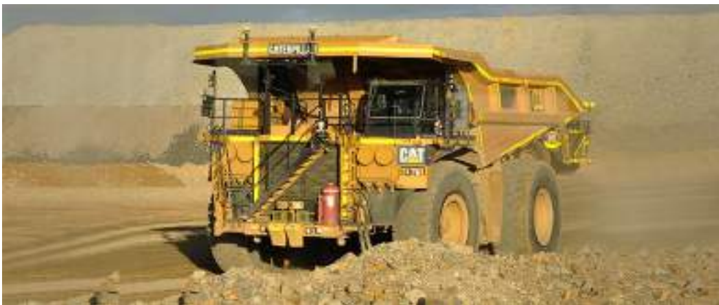
Figure 11. Electric mining truck.
