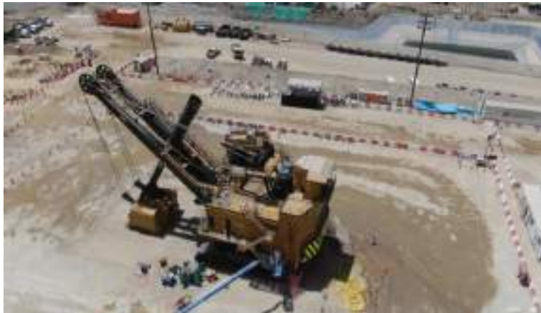
Figure 12. Electric mining shovel.
