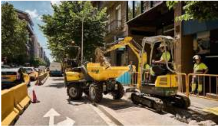
Figure 7. Electrical machinery used in the pilot implementation of electrical machinery in Barcelona manufactured by WackerNeuson.
