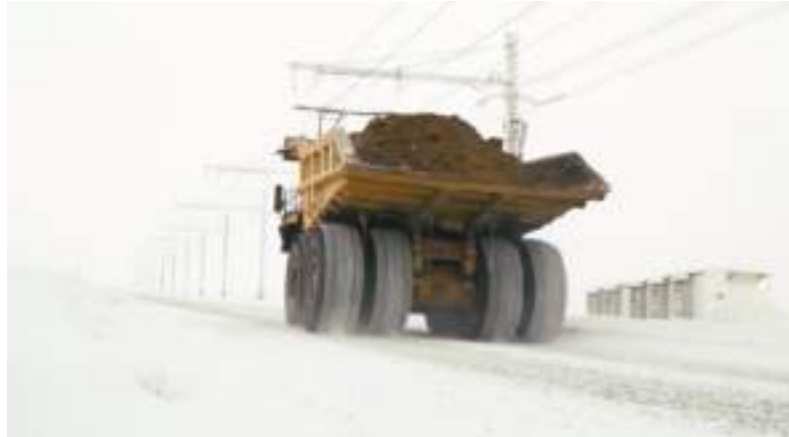
Figure 6. Cat trolley assist system for electrically powered mining trucks.
