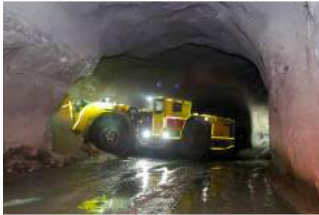
Figure 9. The electric loader in a mining operation demonstration.
