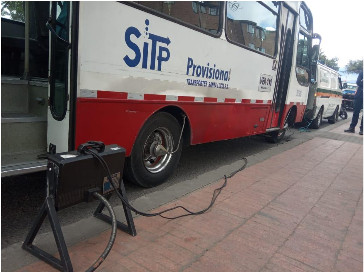
Figure 4: Smoke meter of the District Secretary of the Environment of Bogota, connected to a public transport unit.
