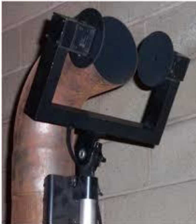
Figure 7: SAE J 1667 smoke meter (full-flow to open-chamber)
