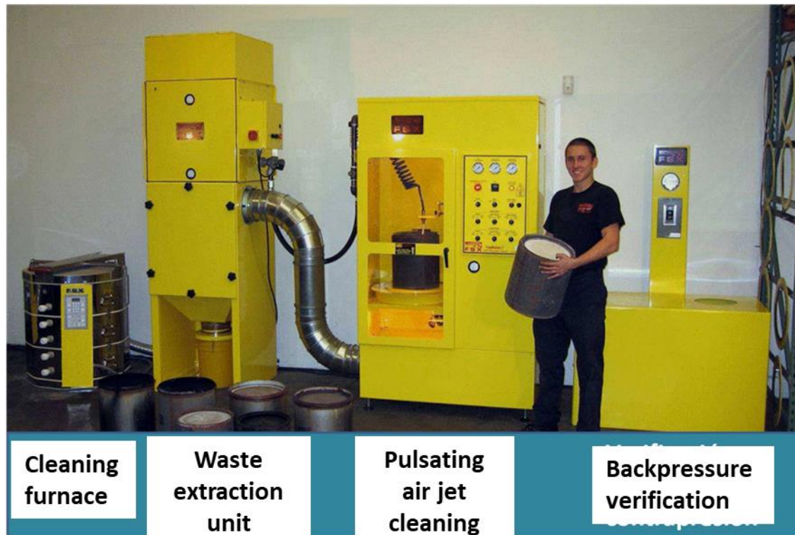
Figure 24: Components of a filter cleaning system
