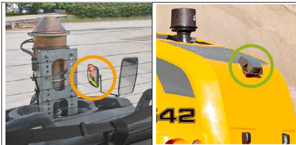
Figure 22: Mirror or camera systems that help to solve visibility problems caused by DPF installation.
