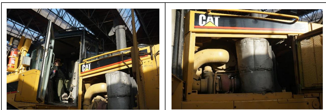
Figure 18: Caterpillar D8R bulldozer part of the Chilean Ministry of Public Works fleet, retrofitted with DPF.
