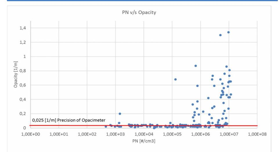
30% of opacity results were close to 0 [1/m] (or below 0.025 [1/m]) but with results between 10E+2 to 10E+9 [#/cm3] in PN.
