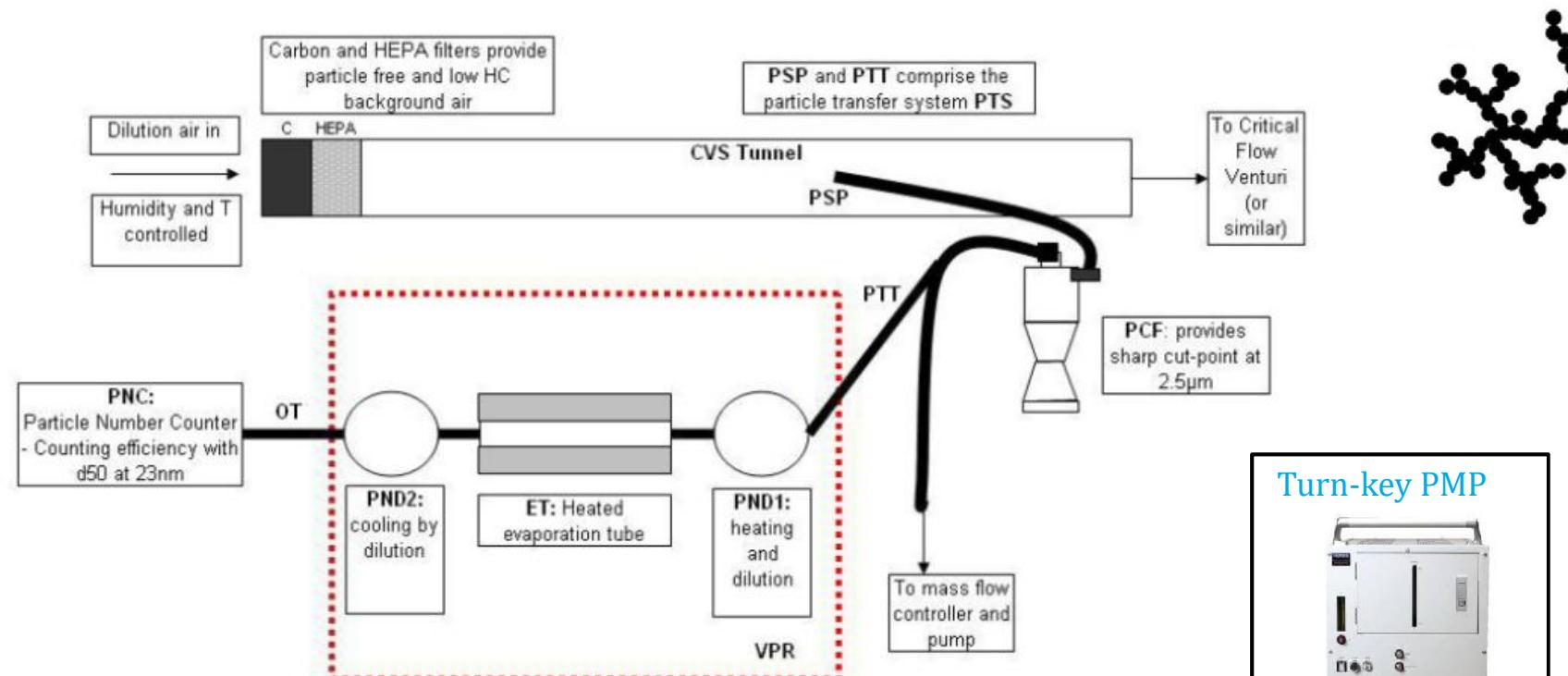
Particle number (PN) legislation implemented by EU based on → Particulate Measurement Programme (PMP) method for solid PN<sup>1</sup>
